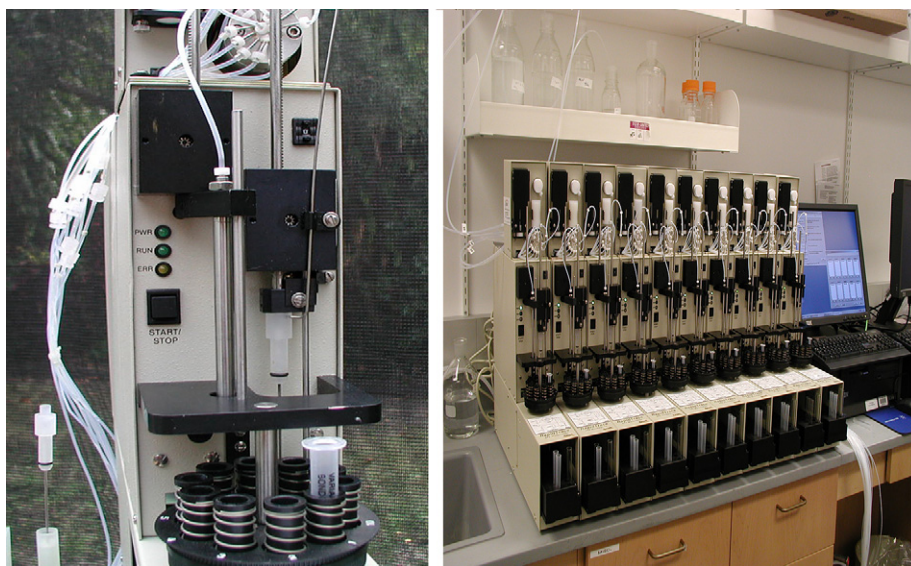
Figure 7. RapidTrace ® SPE workstation (left, single unit; right, 10 parallel units).
